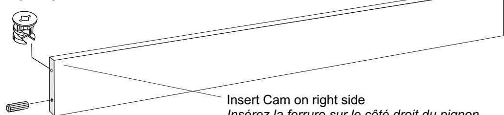
Insert cams in the **unlocked** position, with the opening facing toward the hole for the blue rapid rod.
