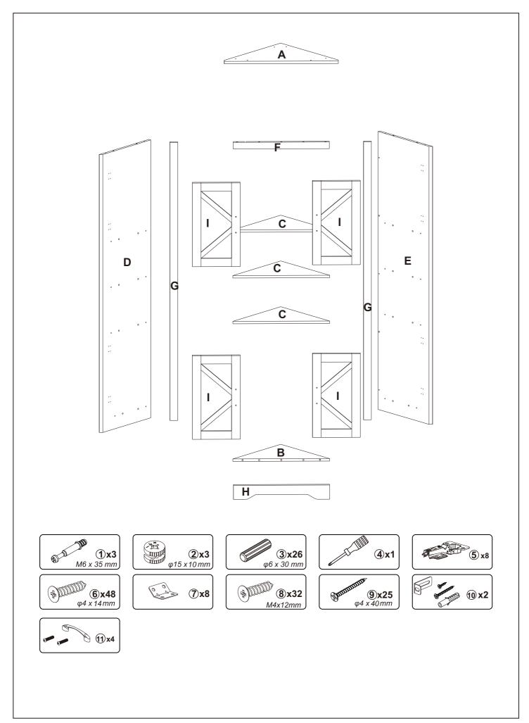
Insert the dowels 3 into part B and C, the installation position is as shown in the figure below.
