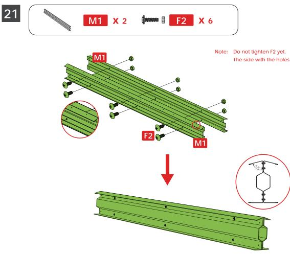
The side with the holes should face upward.
