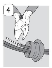
4. Pull cord strain relief out of endbell. Cut green ground wire near the cord strain relief.
