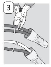
3. Using wire cutters, cut black (or brown) wire and white (or blue) wire near the connectors.
