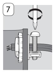
7. Insert the power supply cable, coming from the wall junction box, through the strain relief connector. Tighten connector.
