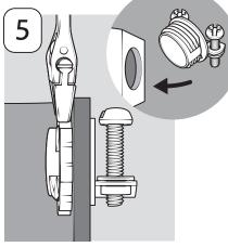
5. Insert metal strain relief connector (not included) into the endbell hole and tighten the nut securely.
