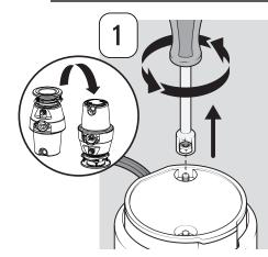
1. After turning off power supply, unbolt two nuts and remove end plate.
