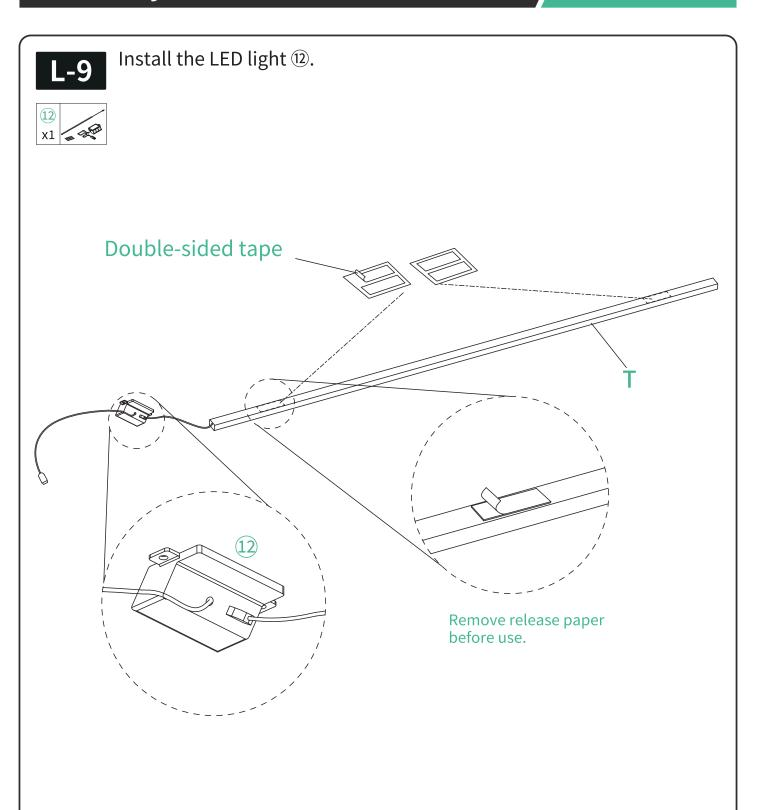
Connect the light strip cable to the socket on the light strip controller as shown in the figure.
