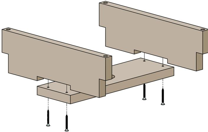
**Note:** The bottom support board should *\*NOT\** sit flush with bottom of the side supports:
