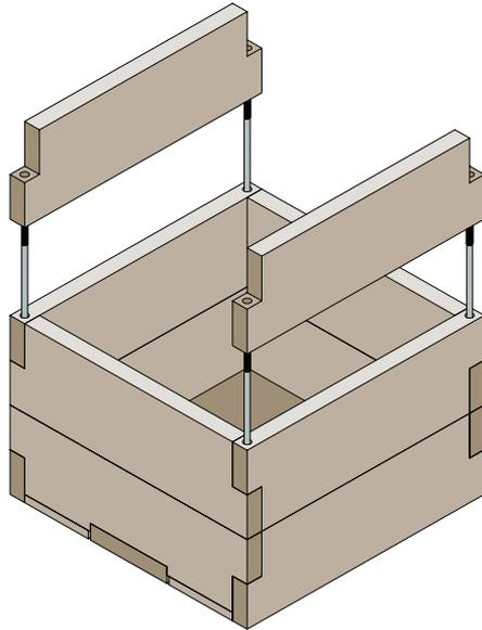
9. Screw the middle pole support board to the pole support side boards – it should fit flush with the notch.
