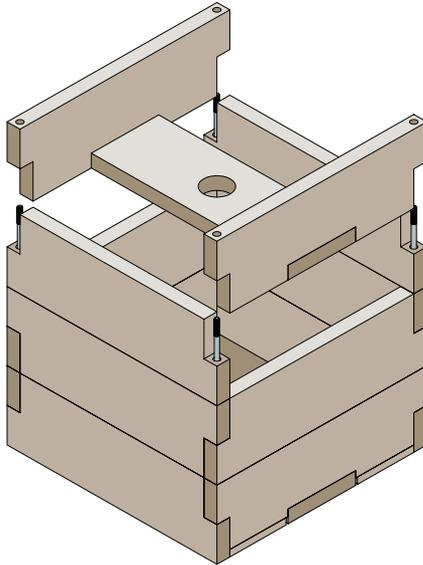
11. Place the bolt caps on top of the rods and tighten using the included allen wrench
