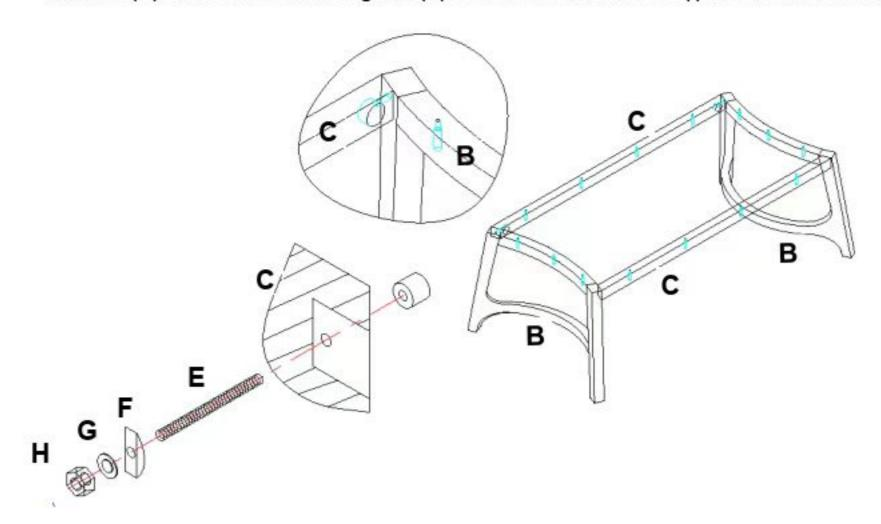
Attach the lower tripod (C) to the foot (B). Use bolts (E), crescent-shaped spacers (F), and flat washers (G) on the holes in the leg rest (C). Screw the Allen wrench (I) into the Allen bolt (H).
