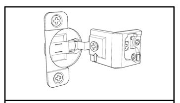
If the door is not level when it is installed, the customer will need to turn the screw clockwise to extend the hinge or counterclockwise to shorten the hinge.
