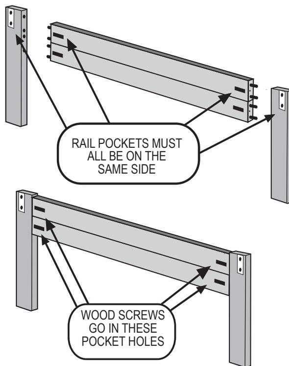
Use a phillips screw driver to attach the Legs to the Bed End using (4) 1 - 1/2" Wood Screws (Black) (H-20).
