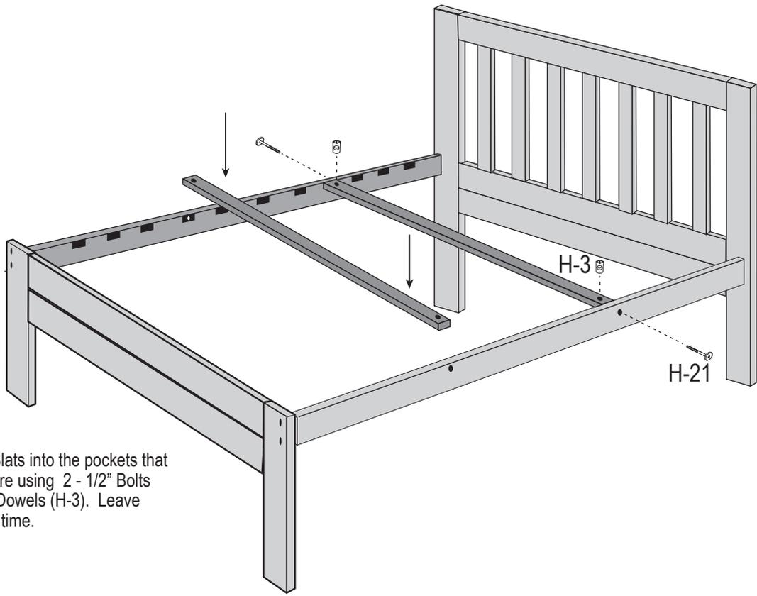
Insert Connector Slats into the pockets that have holes. Secure using 2 - 1/2" Bolts (H-21) and Cross Dowels (H-3). Leave these loose at this time.
