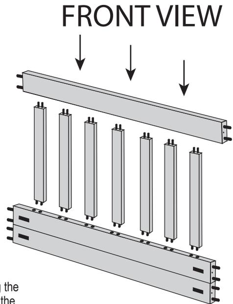
Assemble the headboard by pushing the (7) Headboard Pickets into holes on the Headboard Bottom. Then push the Headboard Top down onto the pickets
