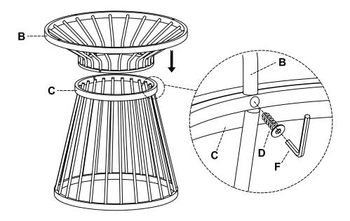
Assemble Base (B/C) to the Top (A) and using the Bolt (E) by Allen Wrench (F). Then through the leveler on the bottom of Lower Base (C) to reach the aim of keeping balance of the product.
