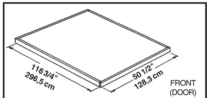
Note: Finished Slab dimensions, with lumber removed.
