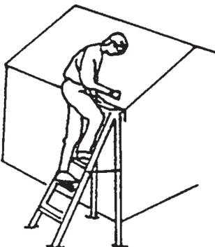
•Do not attempt to assemble the building on a windy day, because the large panels acting as a "sail", can be whipped about by the wind making construction difficult and unsafe.
