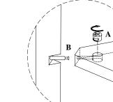
1.) Screw Cambolts ( B ) into Legs ( 3 ). and Place Cam Locks ( A ) into Bottom Panel ( 2 ). \*\*Arrow On Cam Lock Faces Outward Opening \*\*\*\*
