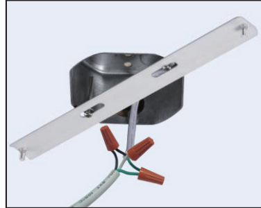
Step 2 1. Connect live supply wire (A) (typically black or the smooth, unmarked side of the two-conductor wires) to live fixture lead (B) with appropriately sized twist-on connector. 2. Connect neutral supply wire (C) (typically white or the ribbed, marked side of the two-conductor wires) to neutral fixture lead (D). 3. For positive grounding in a 3-wire electrical system, fasten the fixture ground (E) (typically copper or green plastic coated) to the fixture mounting strap (1) with the ground screw (2).
