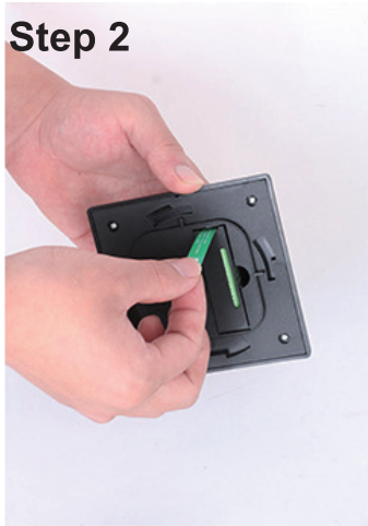
Step 2 Take out the PC insulator and turn on the power button
