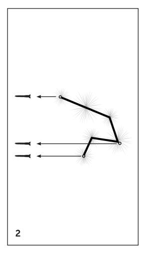
Place three screws into the wall surface.
