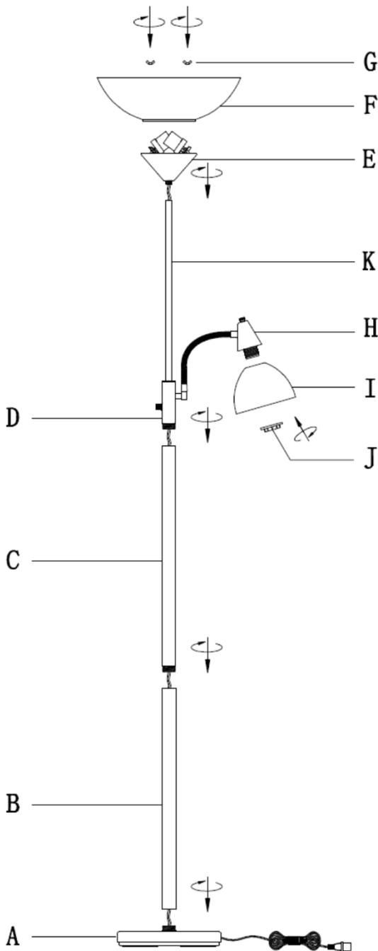
1. Screw the pole (B) onto the base (A) clockwise and screw poles (B), (C) and (D) together until tight. You may need to pull any excess cord gently through the poles so that these two parts fit.
