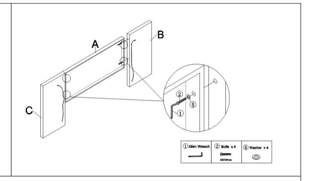
Fix the side headboard (B/C) to the headboard (A) with Bolts(2) and Washers(5) by using Allen Wrench(1) .
