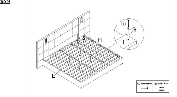
Fix the Slats (L) to the side support bar (H) with Nails(2) by using Allen Wrench(1) or Electric drill.
