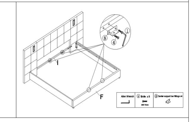
Fix the Center support bar fittings( $\circledast$ ) to the Headboard cross bar( I ) and foot board (F)with Bolts( $\circledast$ ) by using Allen Wrench( $\circledast$ ).
