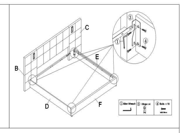
Fix the side rails (D/E) to the side headboard (B/C) and footboard (F) with Bolts(4) and Hinges(3) by using Allen Wrench(1).
