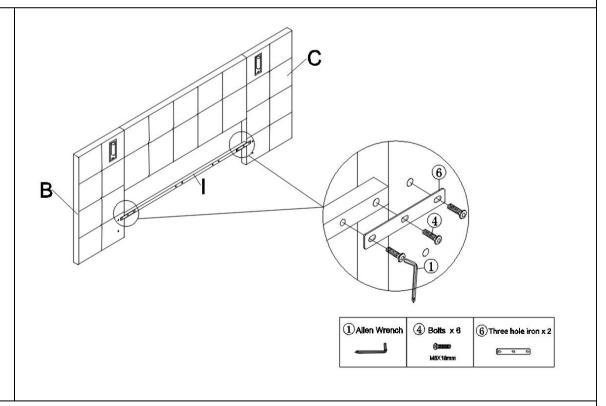
Fix the headboard cross bar ( I ) to the side headboard (B/C) with Bolts (4) and Three hole iron(6) by using Allen Wrench(1).
