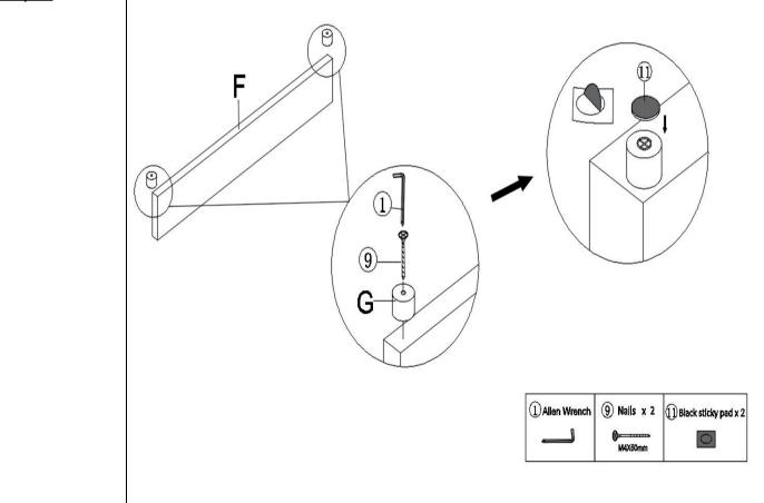
Fix the legs (G) to the Footboard (F) with Nails(③)by using Allen Wrench(①)or Electric drill,then fix the Black sticky pad(①)to the leg.
