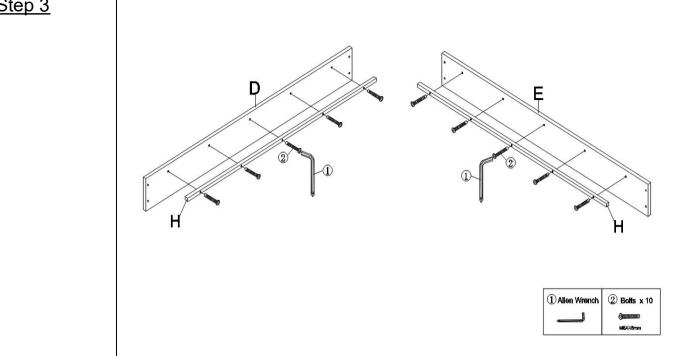
Fix the Siderail support bar (H) to Siderails (D/E) with Bolt(②) by using Allen Wrench(①) .
