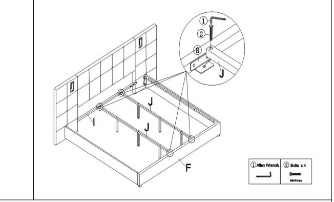
Fix the Center support bar (J )to the headboard cross bar( I )and foot board (F) with Bolts(②) by using Allen Wrench(1).
