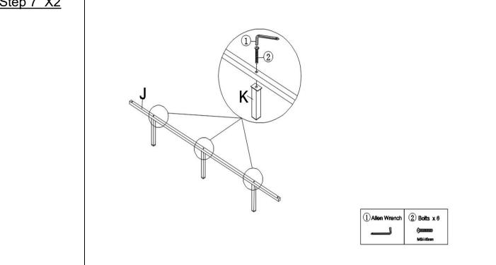
Fix the middle support leg (K) to the center support bar (J) with Bolts(②) by using Allen Wrench(①) .
