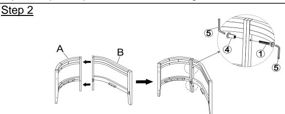
Place the Backrest Panel (A) upright as shown in the picture above onto a clean, soft surface to avoid any scratches or damages to the product. With assistance from your adult partner(s), attach the Left Leg Panel (B) to the Backrest Panel (A) using Bolts(1), Sleeve Nuts(4) and the Allen Key(5) as shown above.
