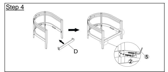
Attach the Support Bar (D) to the assembled frame in step 3 by using Bolts((2)) and the Allen Key((5)) as shown above.
