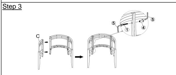
Attach the Right Leg Panel (C) to the pre-assembled in step 2 by using Bolts(1), Sleeve Nuts(4) and the Allen Key(5) as shown above. **Do not fully tighten the Bolts at this time.**
