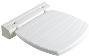
Folding shower seat, manufactured from ABS plastic and structurally reinforced with steel tubing to give it strength and rigidity. Internal friction plates operate the seats lowering and raising safely preventing crashing down. The design uses very little space when in the up position.
