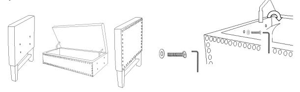
Open the black fabric inside of bench side and use Bolt / Allen Key to fix the legs . Paste back the black fabric
