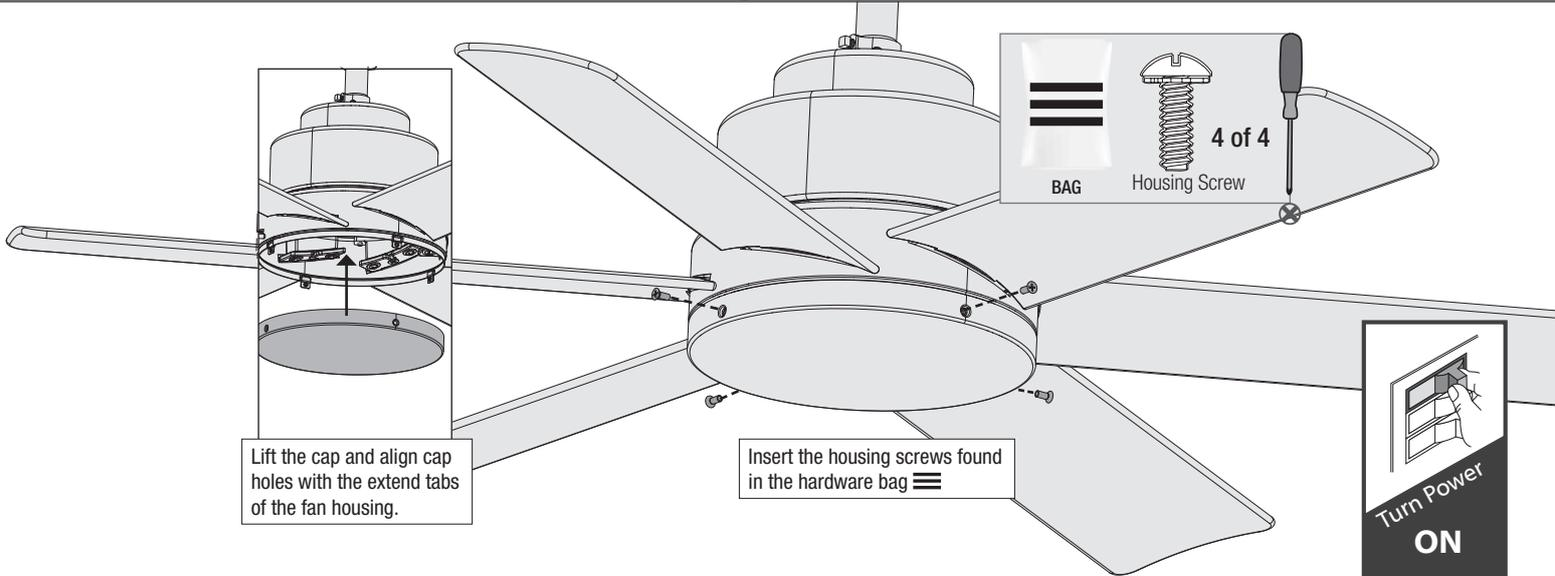
Lift the cap and align cap holes with the extend tabs of the fan housing.
