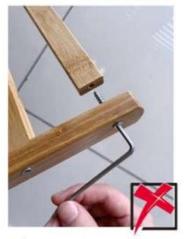
Inserting screws first and then fixing them is incorrect, which may cause damage to the accessories or prevent installation.
