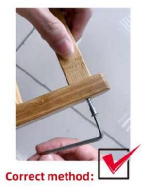
Fix the accessories to align with the hole position, and then tighten the screws, so that they are not easily damaged.
