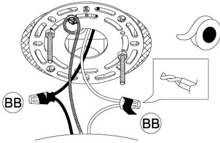
3. Strip 3/8" of insulation from the electrical wire ends. Using wire nuts (BB), connect white fixture wire to the white supply wire from the outlet box; connect the black fixture wire to the black supply wire.
