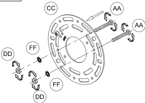
1. Screw screw (AA) onto round mounting plate (CC) and use hex nut (DD) and lock washer (FF) to secure it tight.
