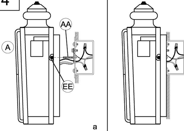
4. Attach fixture (A) to screws (AA) using knurled ball nut (EE) to Secure tightly.
