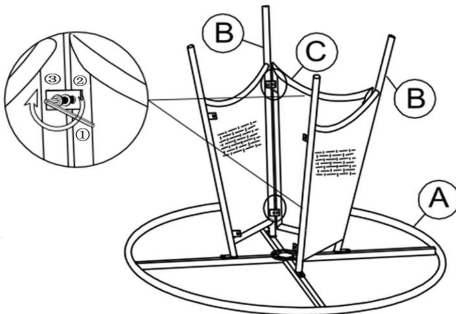
Attach Leg Support Panel (C) between Leg Panels (B) using Bolt (3) and Washer (2) with Allen Key (1) as shown in the picture above.
