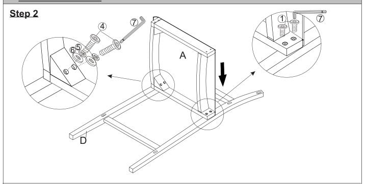
Put the Seat Panel (A) onto Left Leg Panel (D) in the direction of the arrow as shown in above picture.
