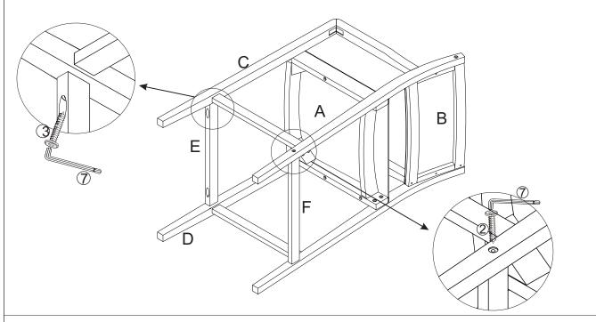
Attach the Right Leg Panel (C) to the Front Leg Connection (E) and Back Leg Connection (F) using Screw (3), Screw (2) and Alley Key (7). **Do not fully tighten the Screws.**
