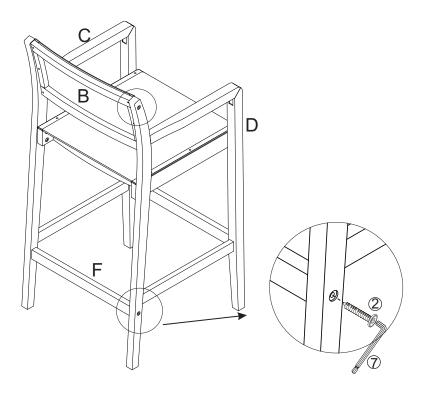
With the assistance of your adult partner, stand the Barstool up. Then secure the Left Leg Panel (D) to the Back Leg Connection (F) and Backrest (B) using Screws (2) and Allen Key (7).
