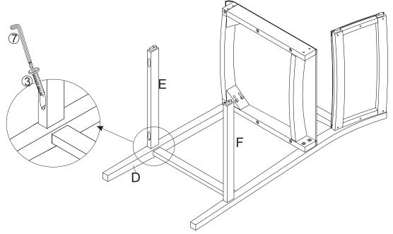
Put the Front Leg Connection (E) and Back Leg Connection (F) onto Left Leg Panel (D). Then attach the Front Leg Connection(E) to the Left Leg Panel (D) using Screws (3) and Allen Key (7).
