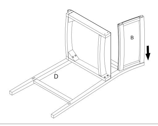
Put the Backrest (B) onto Left Leg Panel (D) in the direction of the arrow as shown in the above picture.
