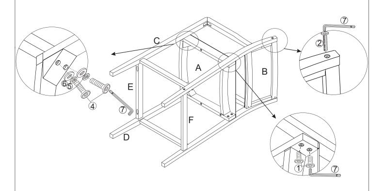
Attach the Right Leg Panel (C) to the Seat Panel (A) using Bolts (4), Bolts (1), Spring Washer (5), Washer (6) and Alley Key (7).
