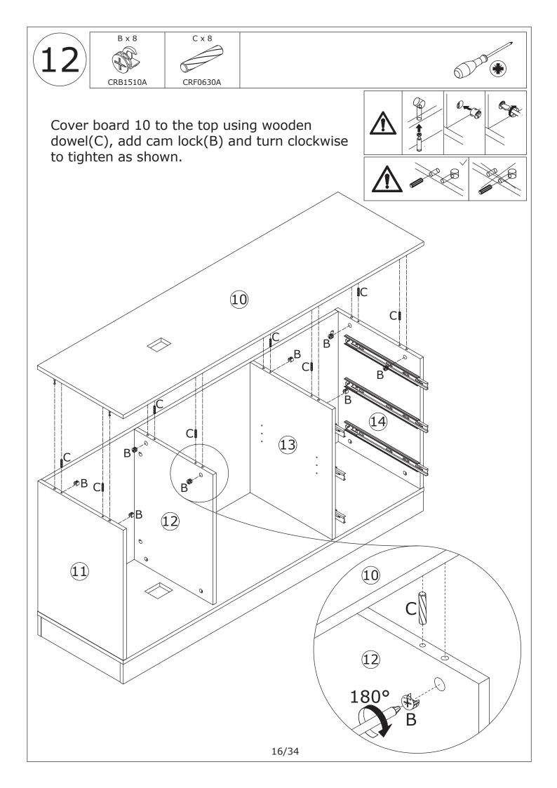
Insert part 2 into the hole of board 10 at first.
