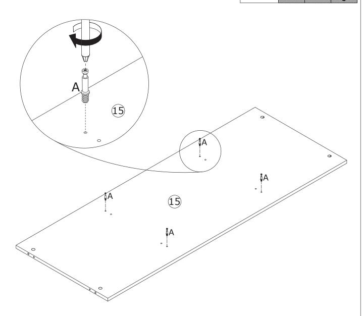
Screw eccentric rod(A) into board 15 as shown.
