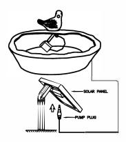
7. INSERT THE SPIKE INTO THE GROUND. POSITION THE SOLAR PANEL TO FACE SOUTH (In Northern Hemisphere) AS MUCH AS POSSIBLE TO MAKE THE MOST OF THE DAYLIGHT HOURS. IT IS IMPORTANT TO ANGLE THE SOLAR PANEL TO FACE SUN WHEN SUN IS AT ITS HIGHEST POINT. ENSURE THE SOLAR PANEL IS NOT SHADED BY TREES, SHRUBS OR BUILDINGS.
