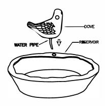
3. ATTACH PUMP TO WATER PIPE, THE PUMP CABLE GET THROUGH OUT FROM A HOLE ON BACK SIDE OF THE RESERVOIR.
