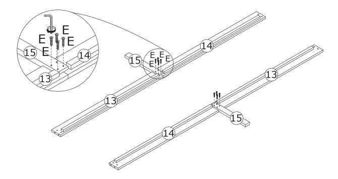
Fix plate #15 to plate #13 and #14 with screw(E) as shown.
