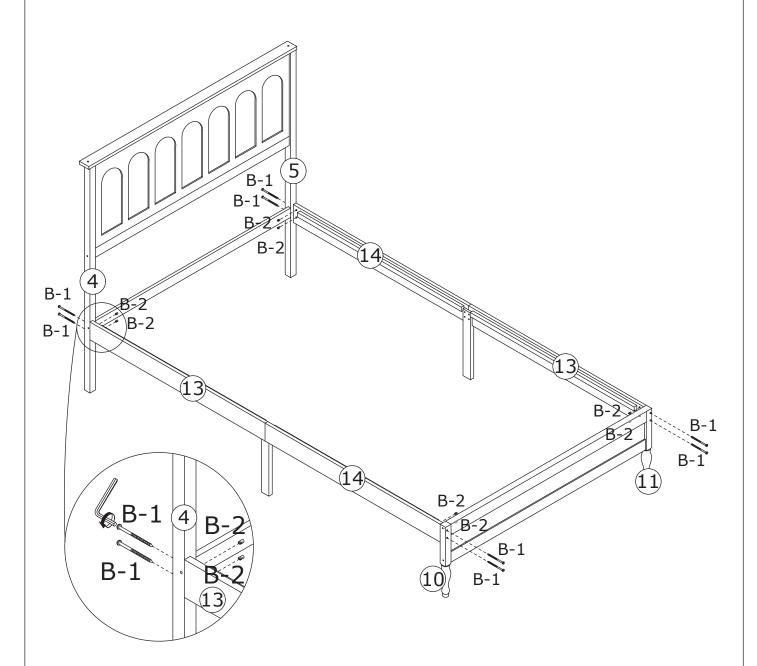
Add nut(B-2) into plate #13 and #14 at first. Fix plate #10, #11 and #4, #5 to plate #13 and #14 with screw(B-1) as shown.
