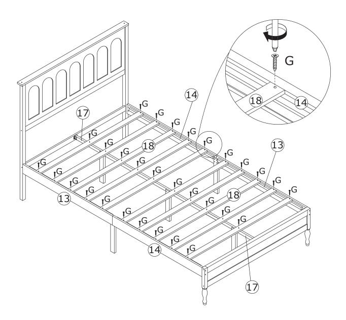
Fix plate #18 to plate #13, #17 and #14 with screw(G) as shown.
