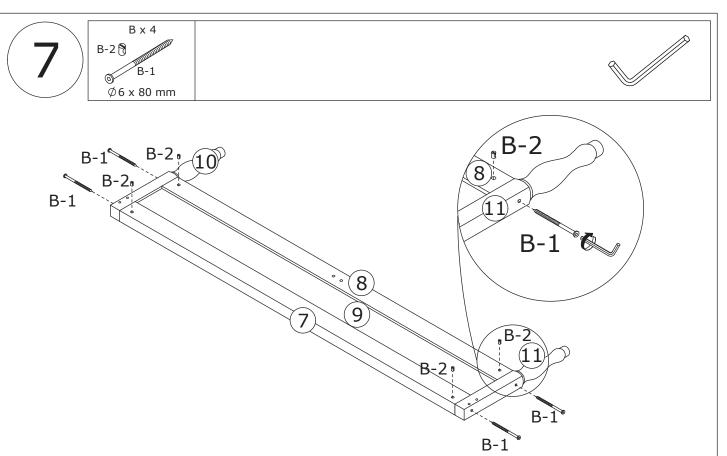
Add nut(B-2) into plate #7 and #8 at first. Fix plate #10 and #11 to plate #7 and #8 with screw(B-1) as shown.
