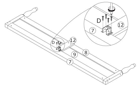
Fix part(D) to plate #7 and #12 as shown.
