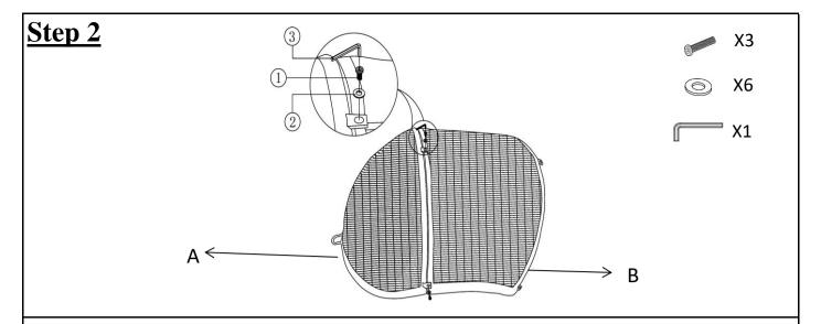
Assemble Top ( A ) and Back ( B ) by using Bolt ( 1 ) and Washer ( 2 )with Allen Key ( 3 ) . Do not tighten.
