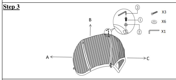
Proceed to assemble Seat (C) and Back (B) by using Bolt (1) and Washer (2) with Allen Key (3). Do not tighten.
