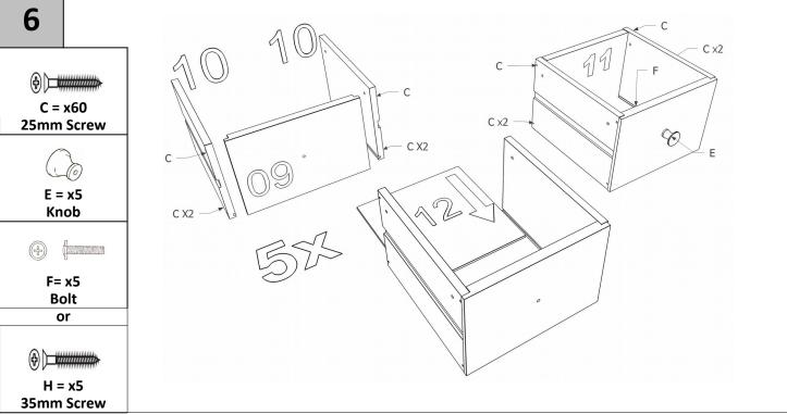
Tip: insert dowels from the inside of the drawers, pushing through so they sit level with the inside of the drawer side.
