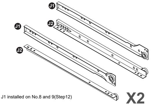
J2 installed on the bottom of the drawer.(Step 29)
