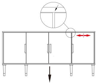
Turn right middle bolt adjuster properly until door is balanced
