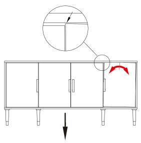
Turn right middle bolt adjuster properly until door is balanced
