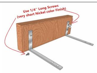
**Optional a)** Line up the metal L-brackets on the pre-drilled holes at the bottom of the small box. You need to screw it in using **¼ inch screws** (very short Nickel color finish)
