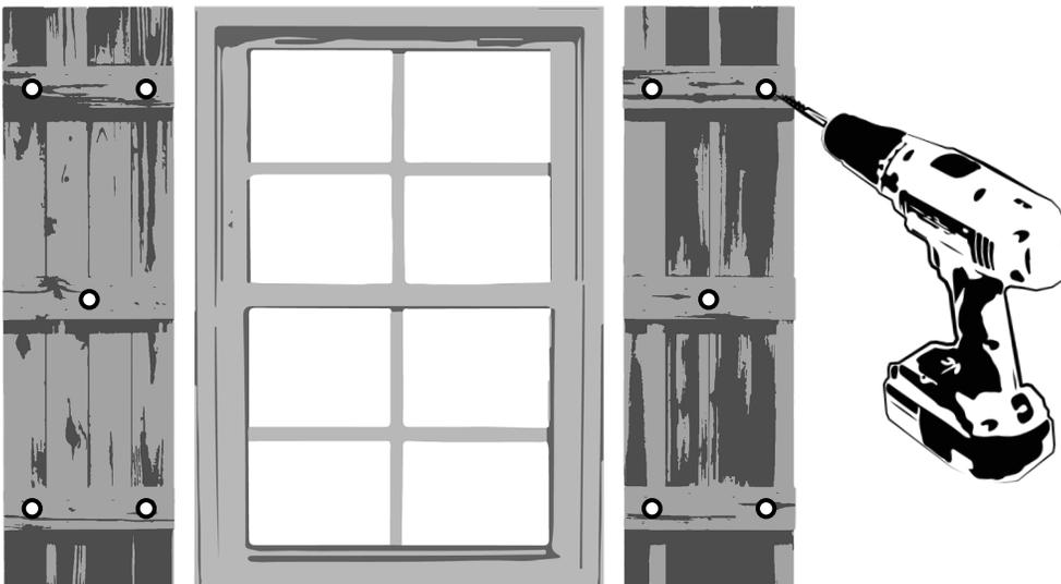
5. Set shutters aside for a moment, and use **1/4" bit** to drill into holes in the wall from the previous step. This will widen the holes in the wall sufficiently to accept wall anchors.
