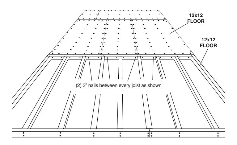
FOR 12 x 24 FLOOR BUILD TWO 12 x 12 FLOORS, ATTACH PRIOR TO INSTALLING FLOOR DECKING
