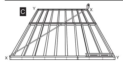
**C:** Completed Floor Frame should be positioned at building site, leveled, using shims between floor frame and ground before proceeding to Floor Panel Attachment.
