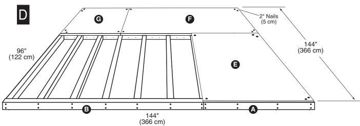
Position Floor Panel 48" x 96" flush to the outside edges of Floor Frame. Position Floor Panel 46-1/8" x 96" flush to the outside edges of Floor Frame. Position Floor Panel 46-1/8" x 48" flush to the outside edges of Floor Frame. Secure panels with two 2" nails at outside corners and one 2" nail at other corners.
