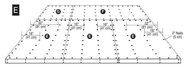
Nails every 12" (30 cm) through Floor Panels into all Floor Bond Boards and Floor Joists
