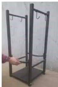
Locate the connector bars and assemble them on the steel frames with hardware.
