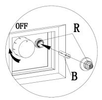
Remove the Electronic Ignitor Cap (16) on the electronic Ignitor (16) by unscrewing and slide the Battery (B) into the battery slot (16).
