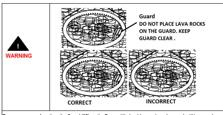
To ensure proper function, the Guard (02) on the Burner (1) should never have lava rocks (A) covered over it.
