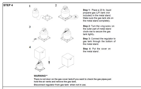
Place the 20lbs Propane Gas Tank (not included) into the Tank cover (09).
