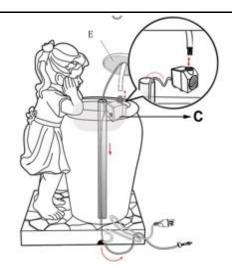
Open the Top(E). Then insert water pipe of the Top(E) into the Pump(C), showed as above.
