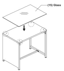
Wipe the suction cups as well as the glass top with an alcohol pad (not included) to ensure there is no dust or debris.
