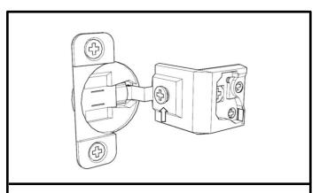
If the door is not level when it is installed, the customer will need to turn the screw clockwise to extend the hinge or counterclockwise to shorten the hinge.
