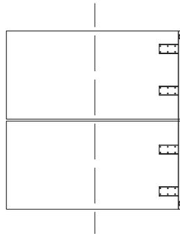
3. Attach hat channels 1/3rd of the way from the front of the worksurface.
