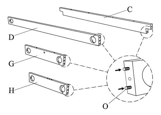
3 Align and fasten Upper Rail(G) and Lower Rail(H) to Turned Leg(B) using JCBB Bolt(M) and Nylon Washer(N) and tighten with Allen Wrench(S).
