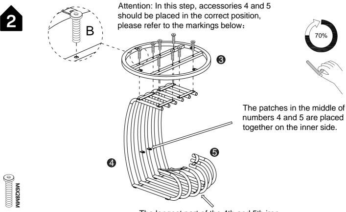
B 8 pcs The longest part of the 4th and 5th iron pipes are pressed together on the inside.
