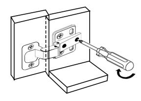
Adjusting screws can change the gap between the door panel and the cabinet side
