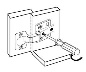
Adjusting screws can change the door panel relative to the cabinet next to the coverage
