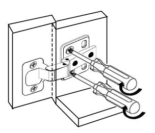
Adjusting screws can correct the upper and lower clearance of the door panel
