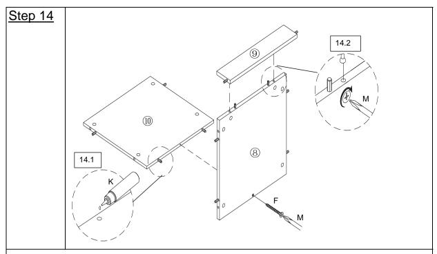
**14.1)** Apply Glue (K) into the mounting positions on Bottom Panel 8 and Support Panel 9.
