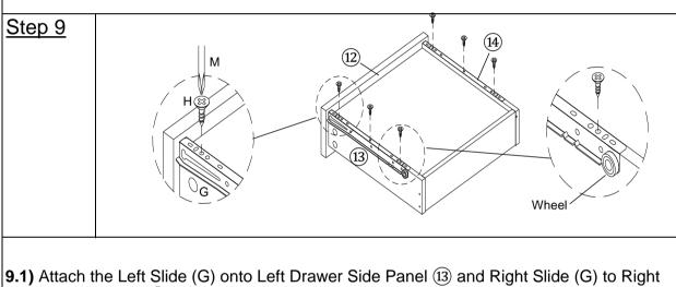
Drawer Side Panel (4) using Screws M4 x 12mm (H) and screwdriver (M). Caution: Make sure the drawer rail (G) touches Drawer Front (12). Note: There are pre-existing mounting positions on the Panels to attach the Drawer Slides (G).
