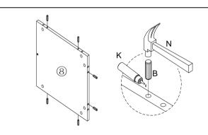
**2.1)** Apply Glue (K), and insert Wood Dowels M8x25mm (B) into the mounting positions on the
