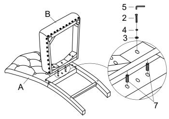
STEP 2: Assemble the cushion seat (B) with the back legs of the chairback (A) by using Allen Key (5) with hardware 1,3, and 4.
