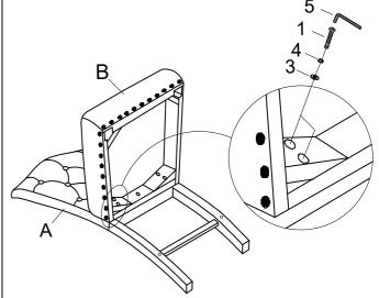
STEP 3: Assemble the front legs (C) with the Cushion Seat (B) by using Allen Key (5) with hardware 1, 2, and 4.
