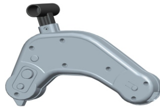
Road Roller/Pushdozer arm
