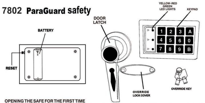
Open the override lock cover, insert the override key and turn counter-clockwise until it stops. Next turn the handle clockwise to open the safe.
