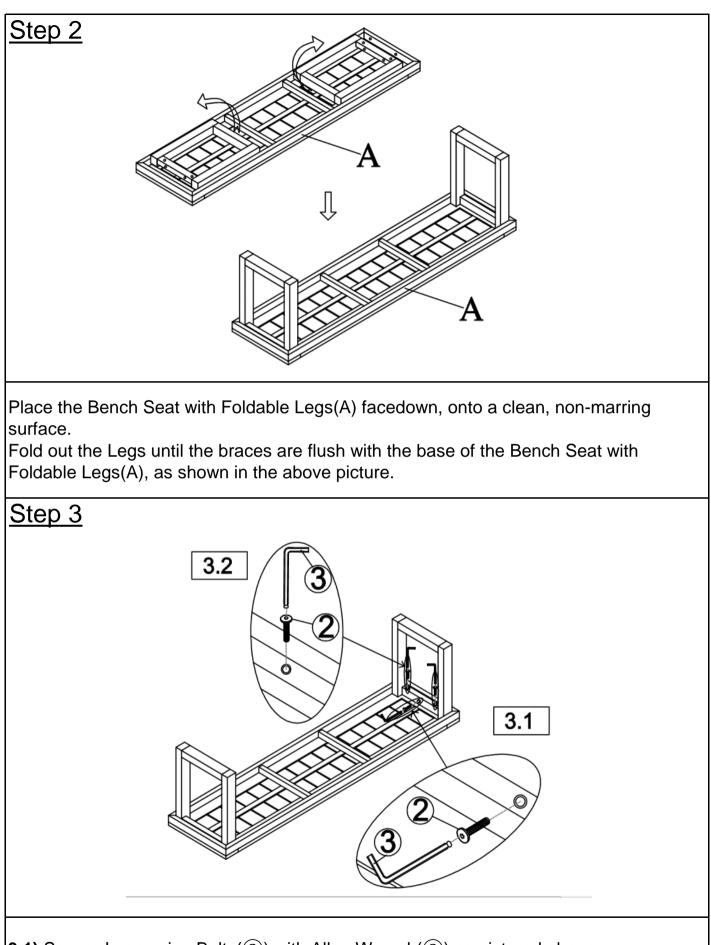
**3.1)** Secure Legs using Bolts(2) with Allen Wrench(3) as pictured above. **3.2)** Secure Legs using Bolts(2) with Allen Wrench(3) as shown above. **Do not fully tighten the Bolts.**
