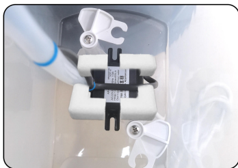
1. Remove the foam around the pump
